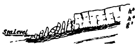
FIG. 39 a .—Section of the landslip of Axmouth, Devon. h^a =Lias clay; h^b =Greensand; h^c =Chalk.
